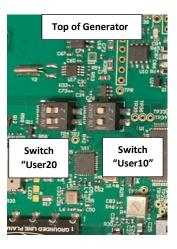
• Collision Avoidance Module Disable – Disables the CAM from providing responses to magnetic fields from other trucks with MFGs installed. With switch "Sw2" in Switch "USER10" set to OFF the CAM is fully functional and set to ON the CAM is disabled.
