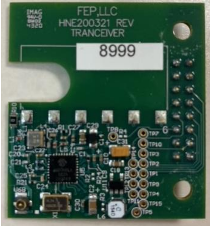
Printed Circuit Board-Top Side RF Board
