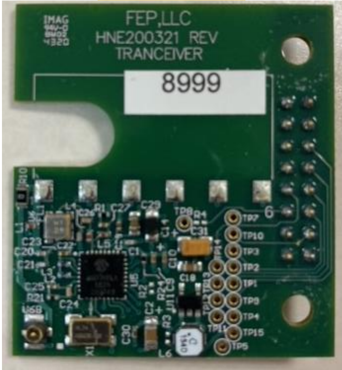
Printed Circuit Board-Top Side RF Board
