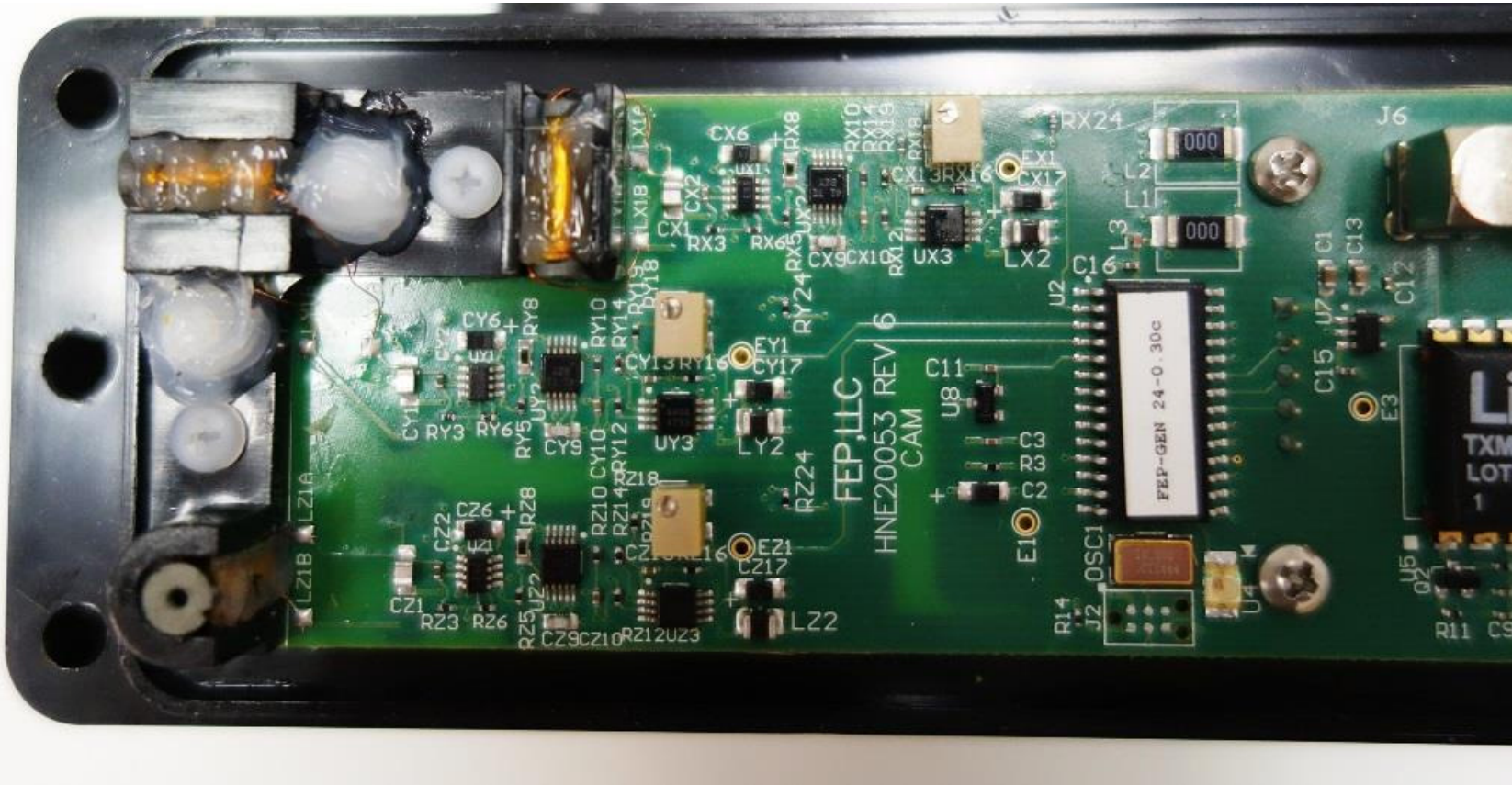
Magnetic Field Generator w/ CAM-Internal Photos Open Middle Housing Collision Avoidance Module Board (pt. 2)
