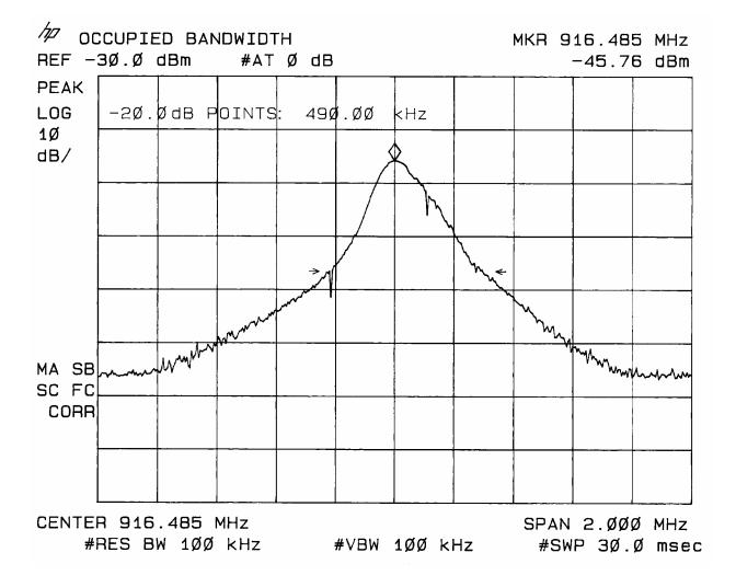
The field strength measurements were taken using an HP8596E spectrum analyzer, an EMCO 3121C dipole set, and an EMCO 3115 double ridge guide horn. The test sample was set to transmit a repeating code pattern and the field was scanned from 30MHz. to 10GHz. All emissions within 20 dB. of the limits were noted.
