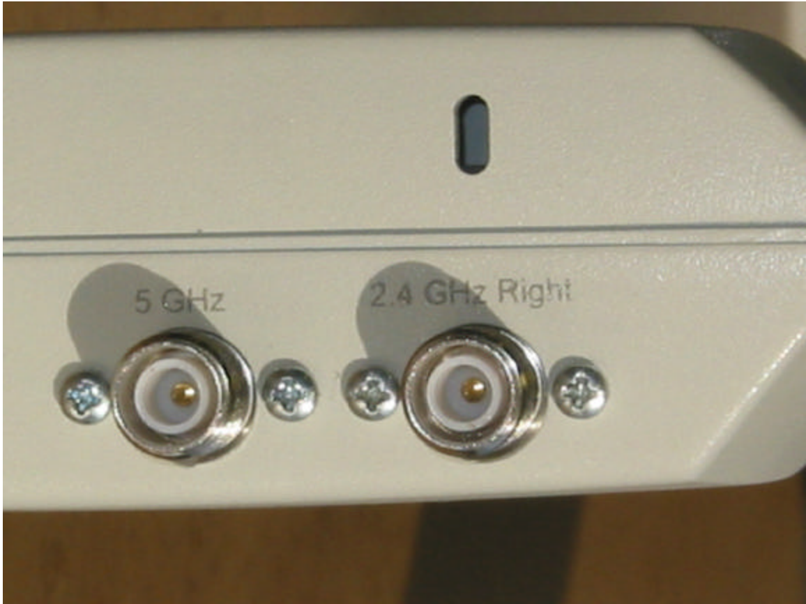
The 5GHz Reverse TNC External connector, (Currently not certified for use and disabled) and one of the reverse TNC external antenna connector for 2.4 GHz
