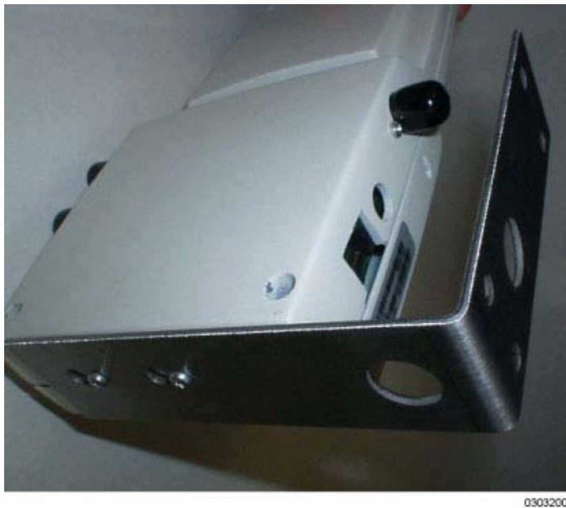
Figure - Assembling the Airespace AP to the Projection-Mount Bracket
