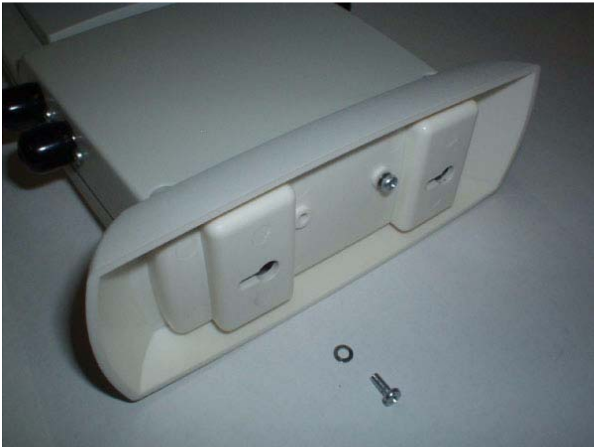
Figure - Assembling the Airespace AP and Ceiling-Mount Base
