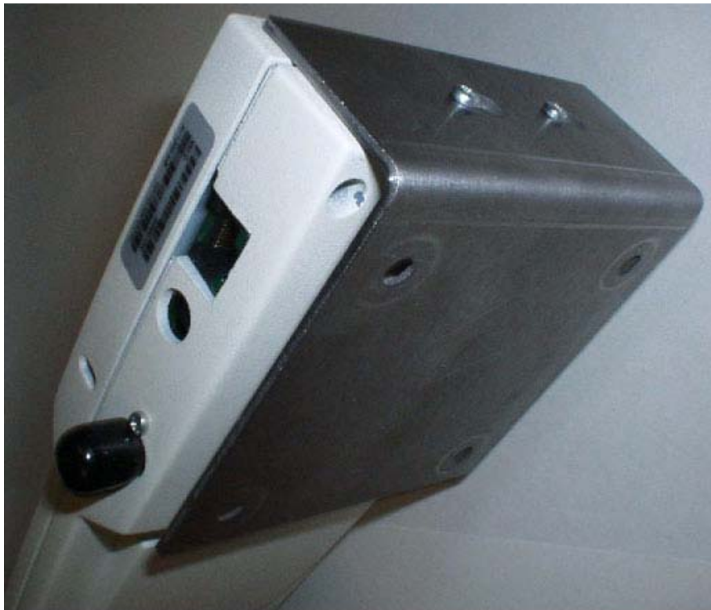
Figure - Assembling the Airespace AP to the Flush-Mount Bracket
