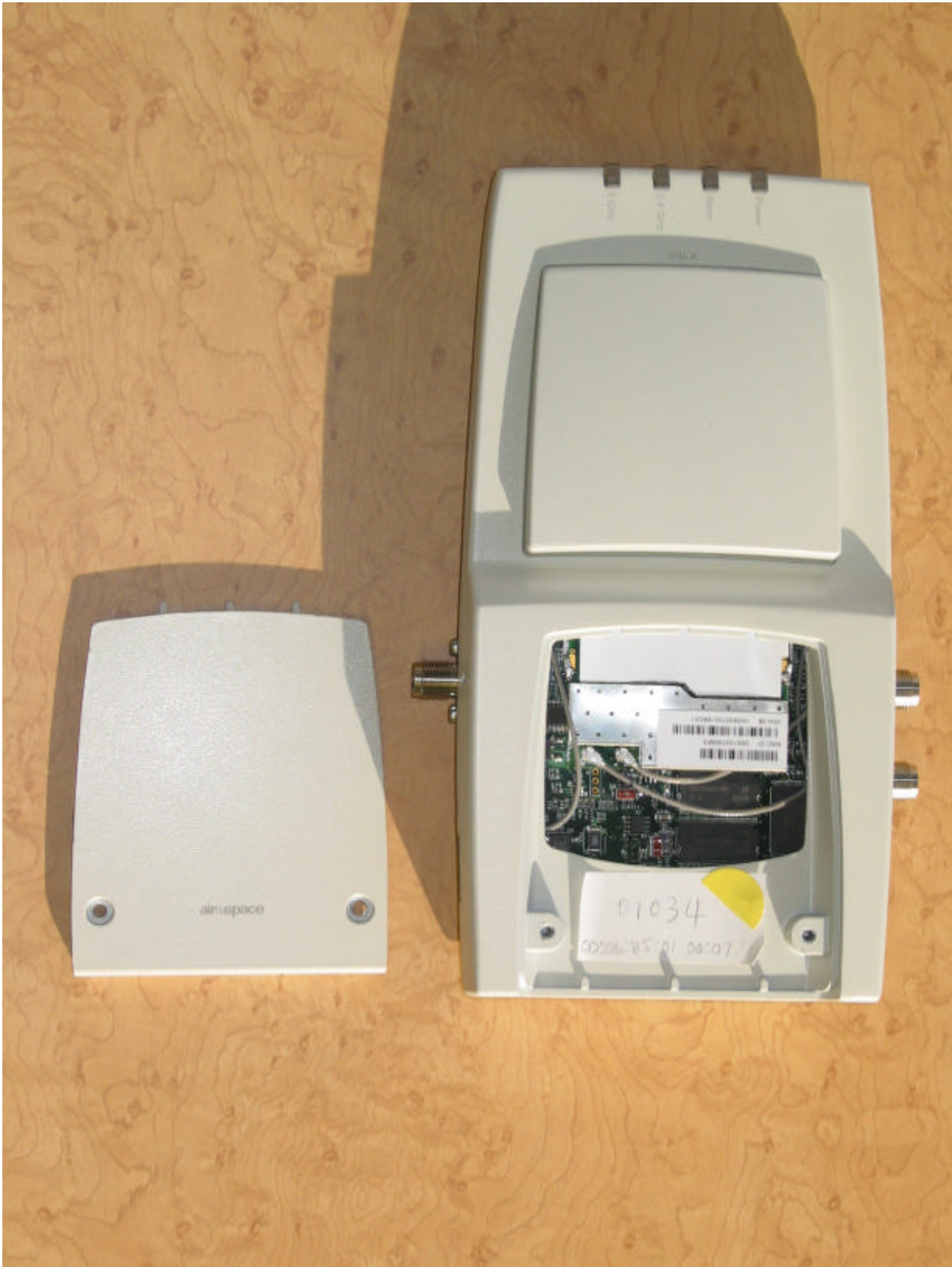
1200A with Access door removed
