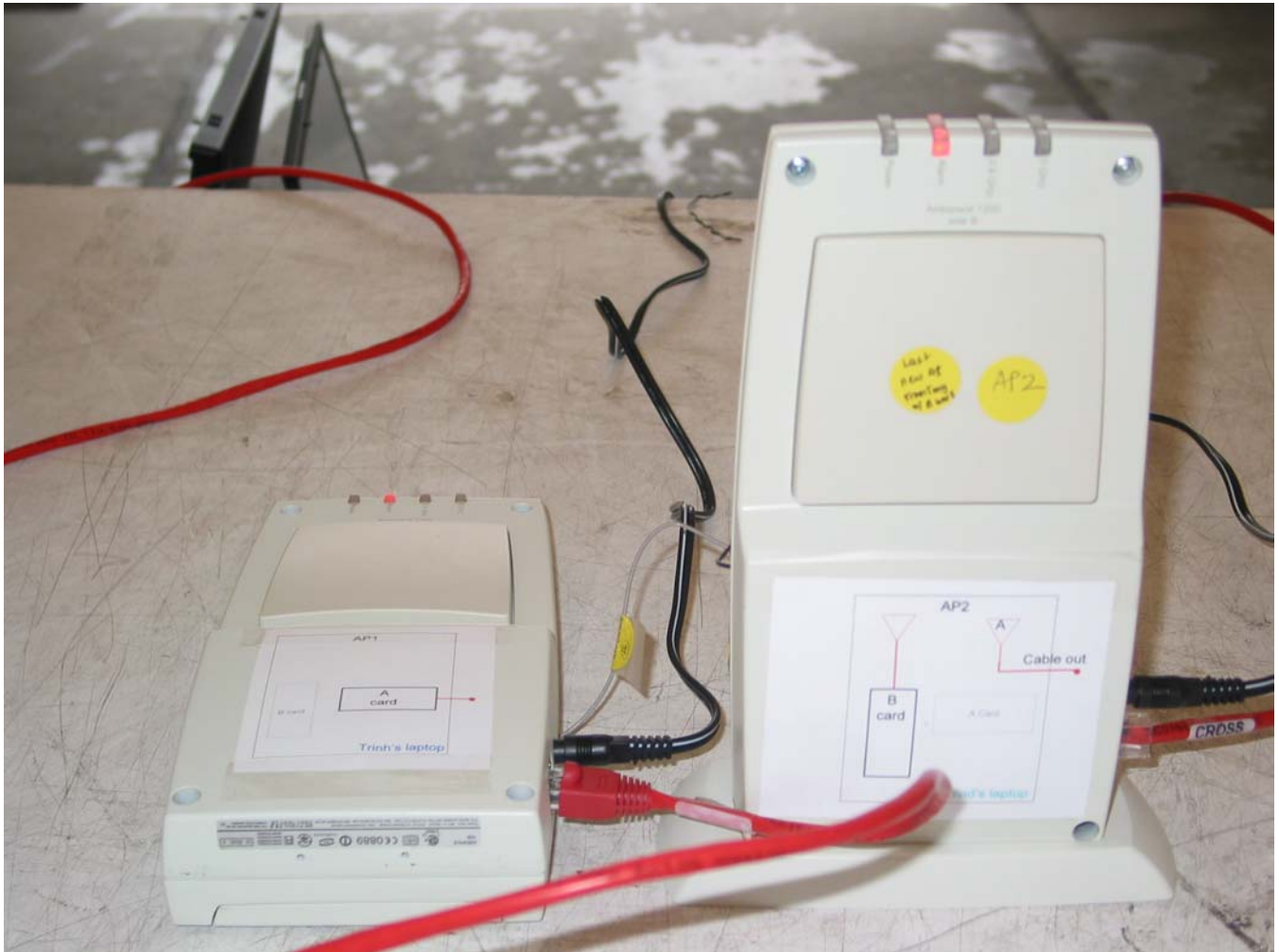
Dual Xmit, Radiated Emissions Test Setup (One unit is laying on its side so as to not interfere with the radiating pattern of the antennas in the unit that is standing.)
