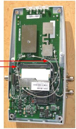
These cables connect the main PCB to the external 2.4 GHz antenna connectors
