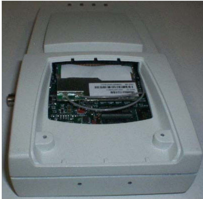
Figure - 802.11a Radio Card Installed in the Airespace AP Case
