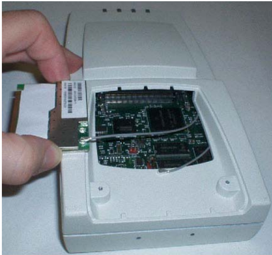
Figure - 802.11a Radio Card with RF Cable "1" Attached
