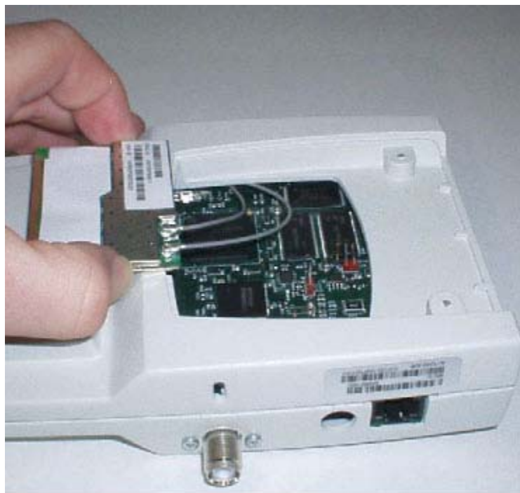
Figure - 802.11a Radio Card with RF Cables "1" and "2" Attached
