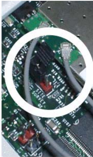
A. Site Survey Jumper Not Installed
