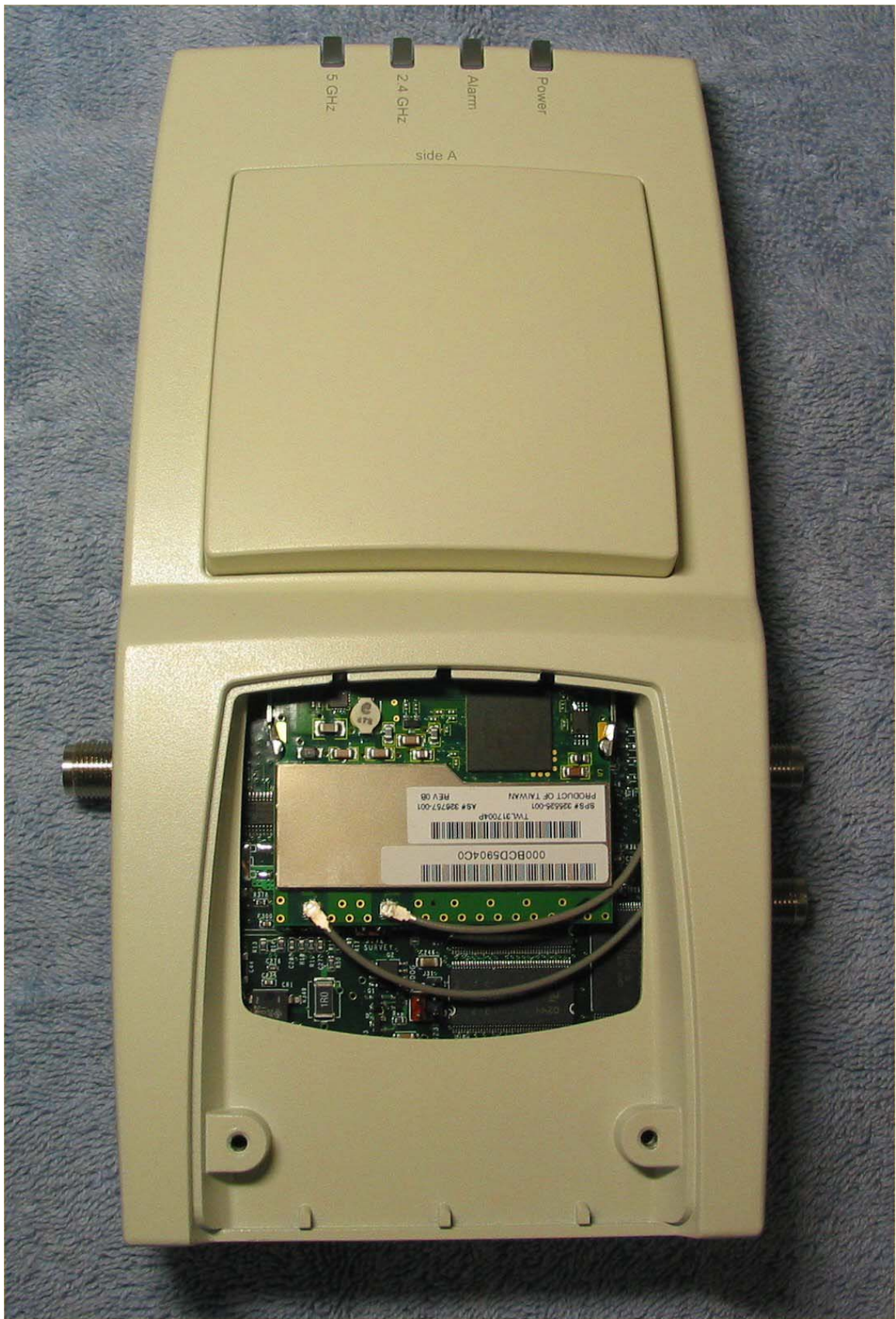
Access point with cover removed
