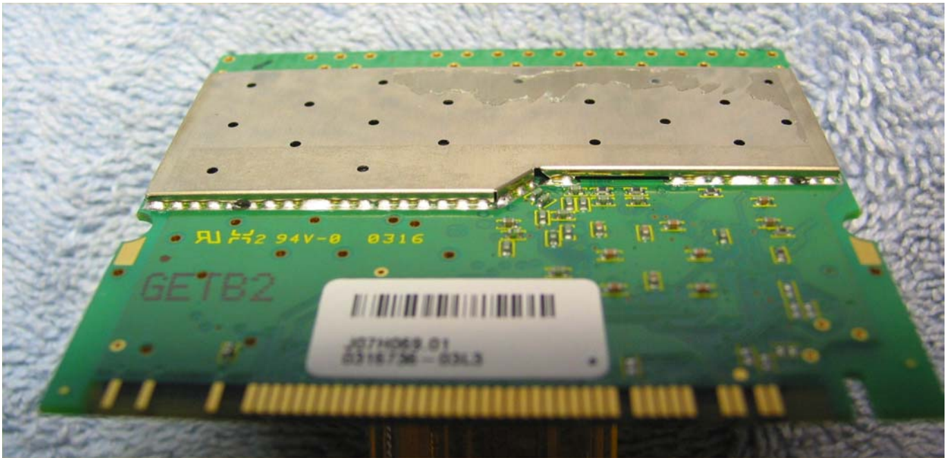
IEEE 802.11 mini PCI module, Rear, label removed Shield soldered, not removable.
