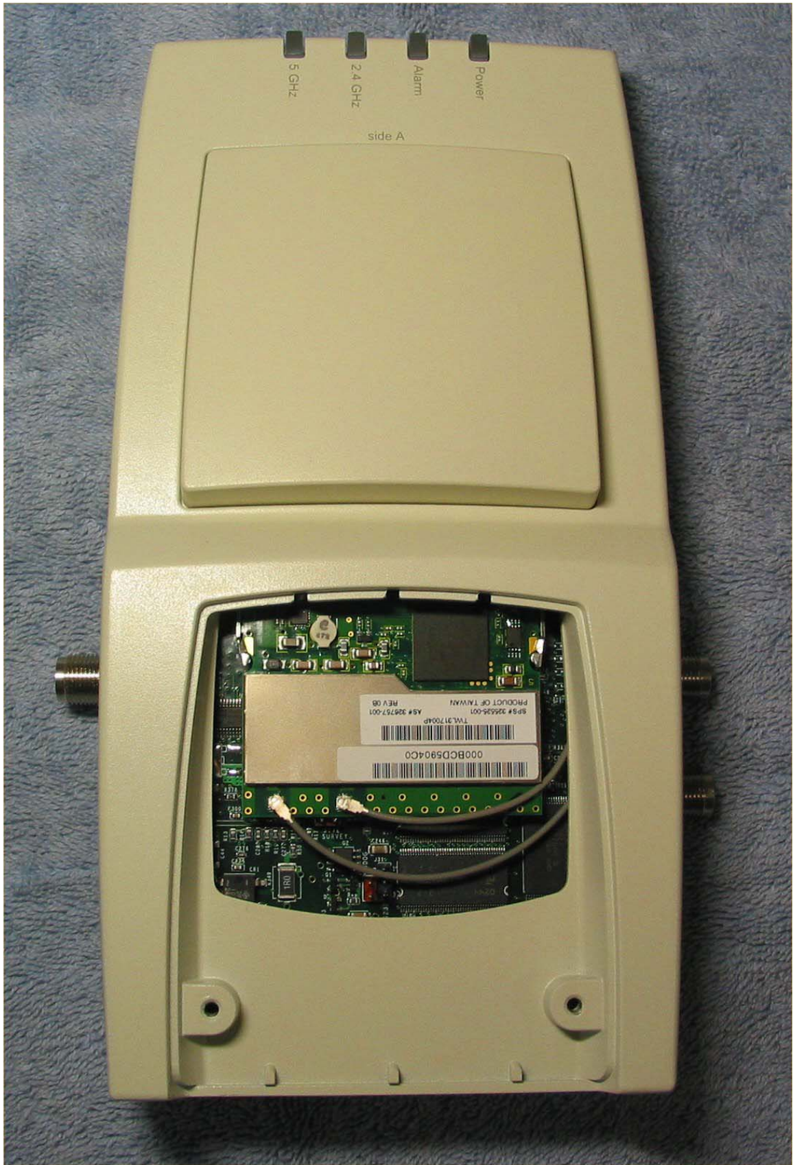
Access point with cover removed
