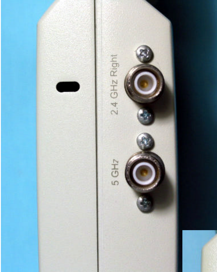
Airespace Access Point, Connector Detail Model 1200
