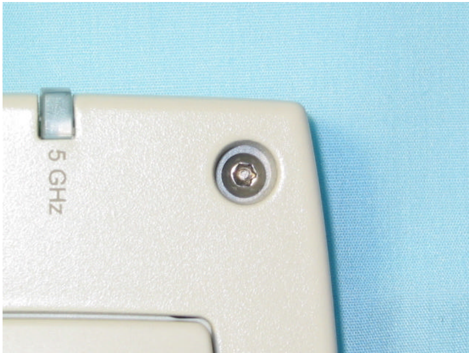
Airespace Access Point, Models 1200 and 1200 INT Security Screw detail
