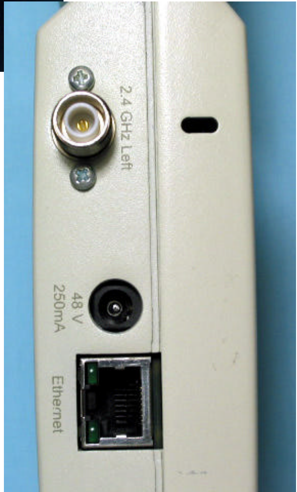
Airespace Access Point, Connector Detail Model 1200
