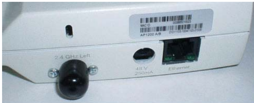
A. 2.4 GHz/802.11b Left External Antenna Port
