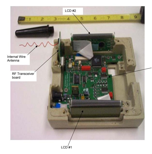
uP board Interface to LCD Display #2
