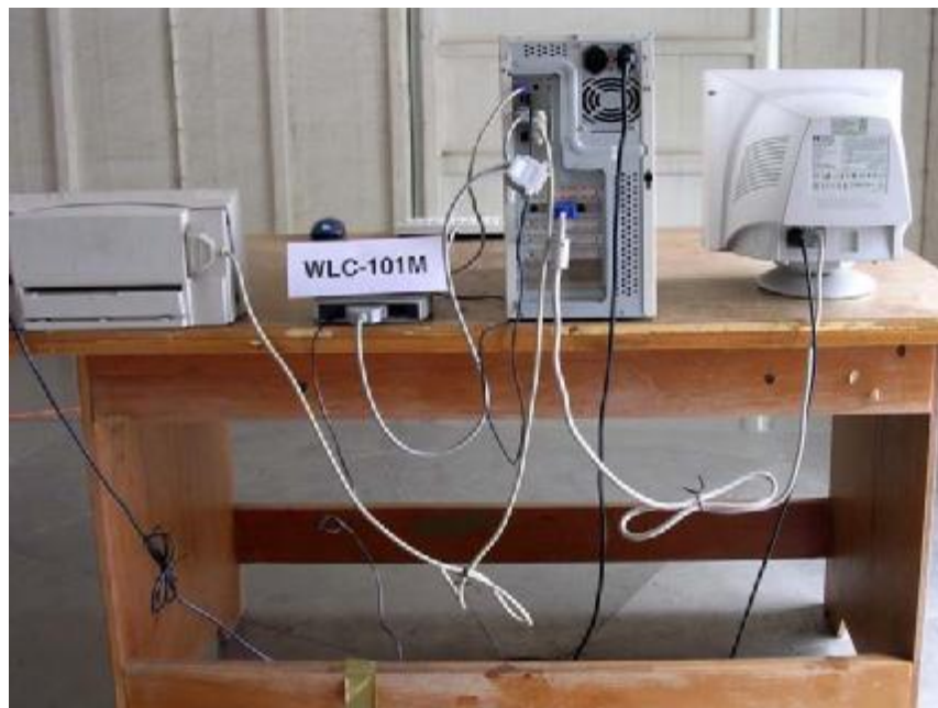
Photo 4: Radiated Emission Test Set-up (rear)
