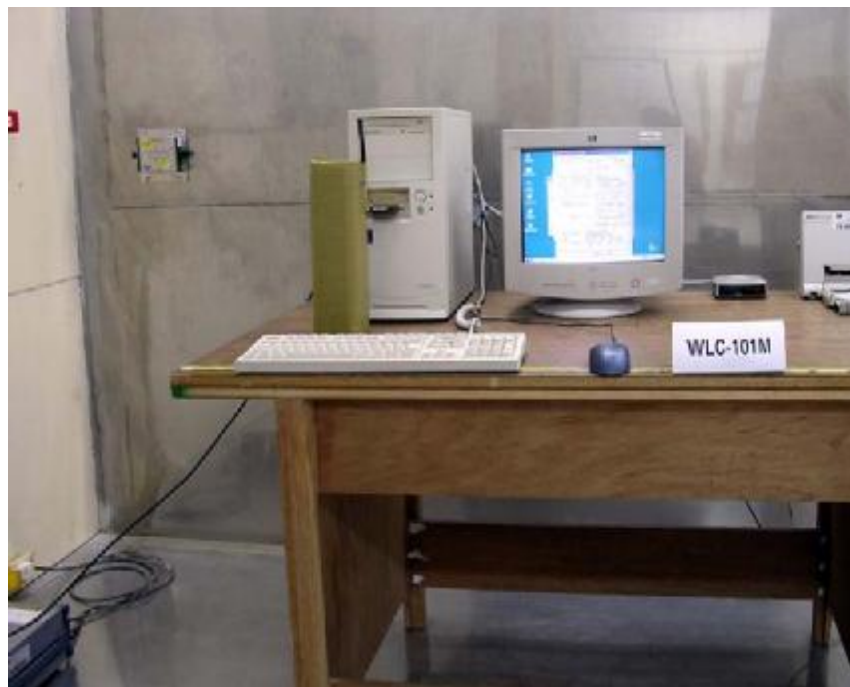
Photo 1: Conducted Emission Test Set-up (front) (EUT with antenna 1)
