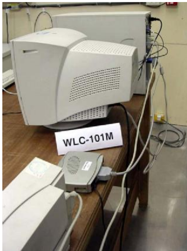
Photo 3: Conducted Emission Test Set-up (rear) (EUT with antenna 1)
