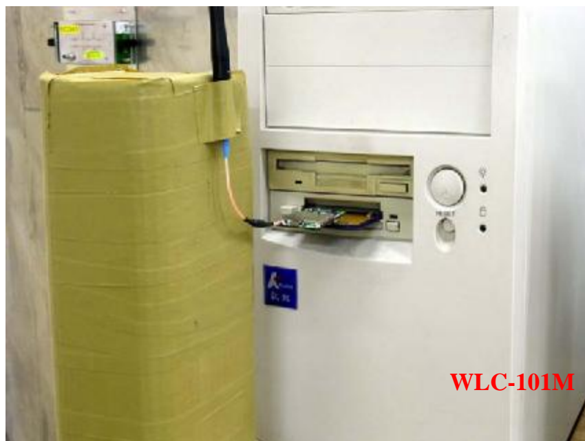
Photo 2: Conducted Emission Test Set-up (front) (EUT with antenna 1)
