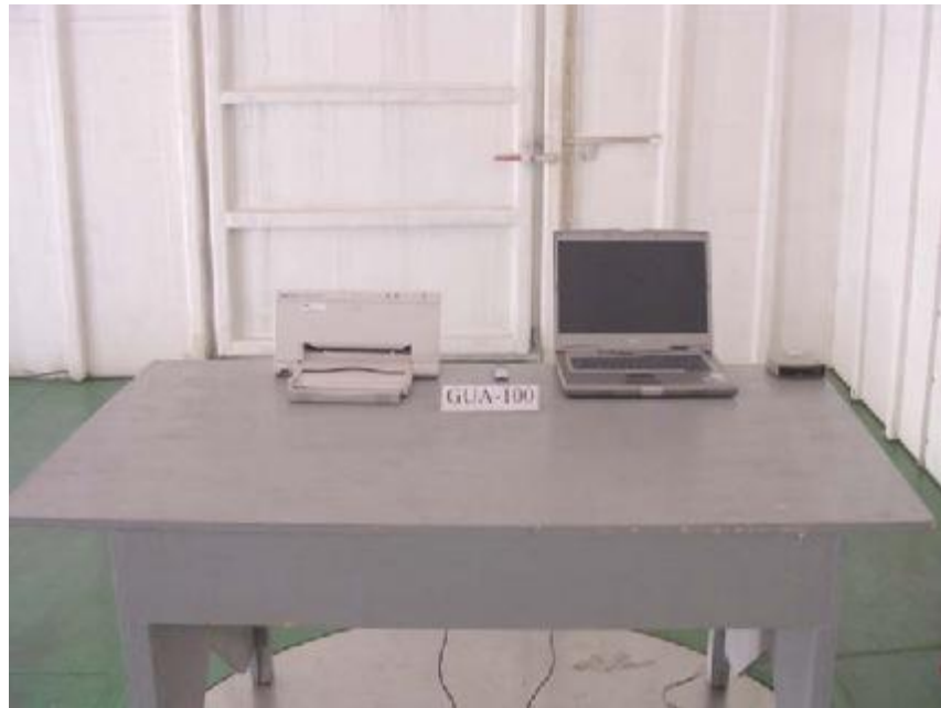
Photo 2: Radiated Emission Test Set-up
