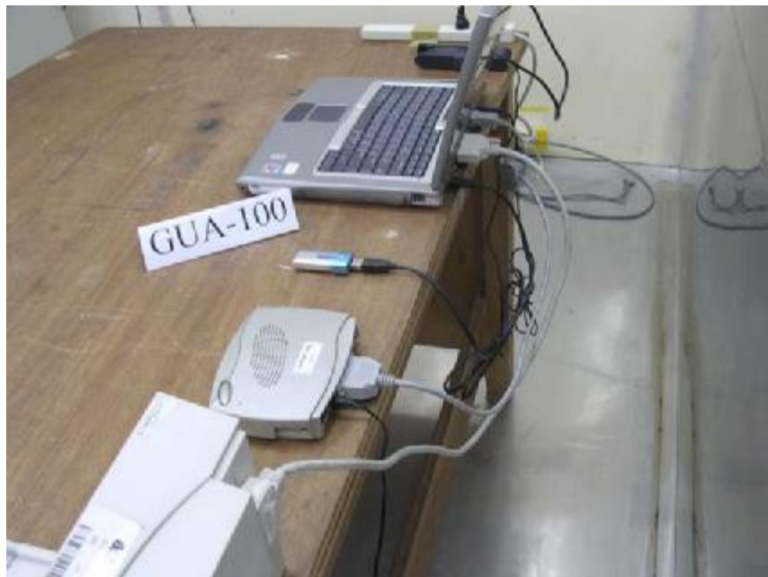
Photo 2: Conducted Emission Test Set-up
