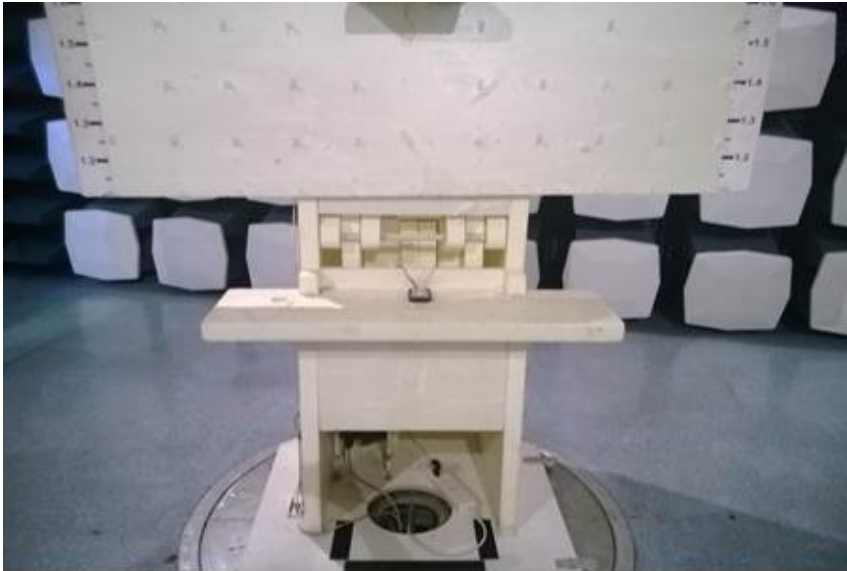
Picture 2. FCC Part 15B Radiated emissions
