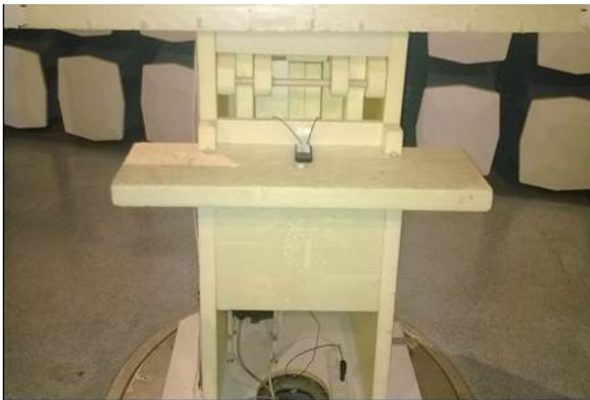
Picture 2. FCC Part 15B Radiated emissions
