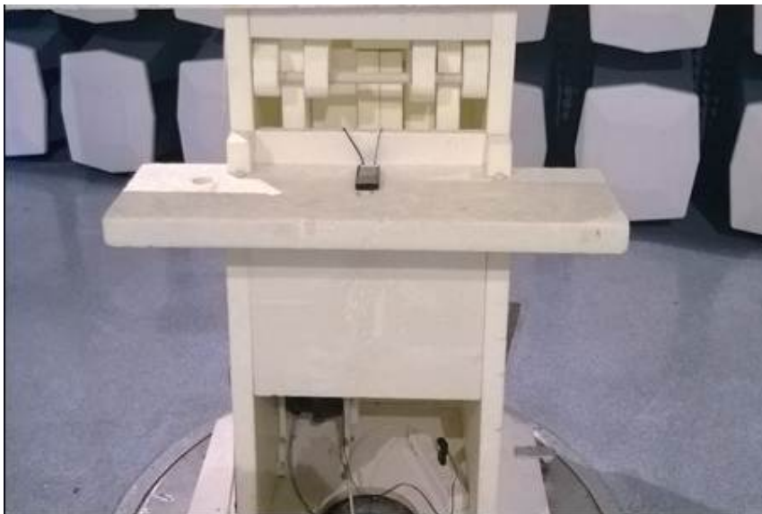
Picture 2. FCC Part 15B Radiated emissions
