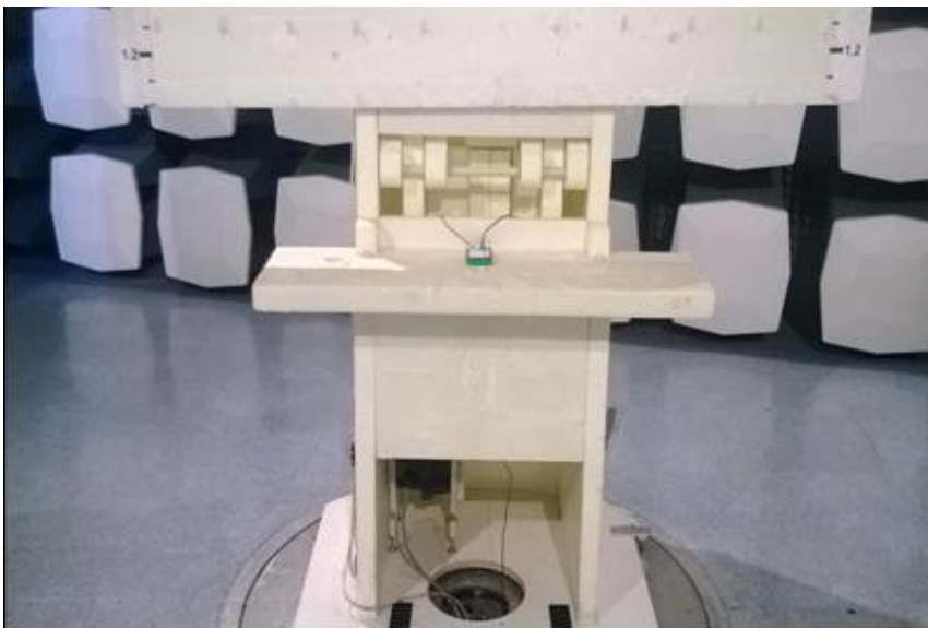
Picture 2. FCC Part 15B Radiated emissions
