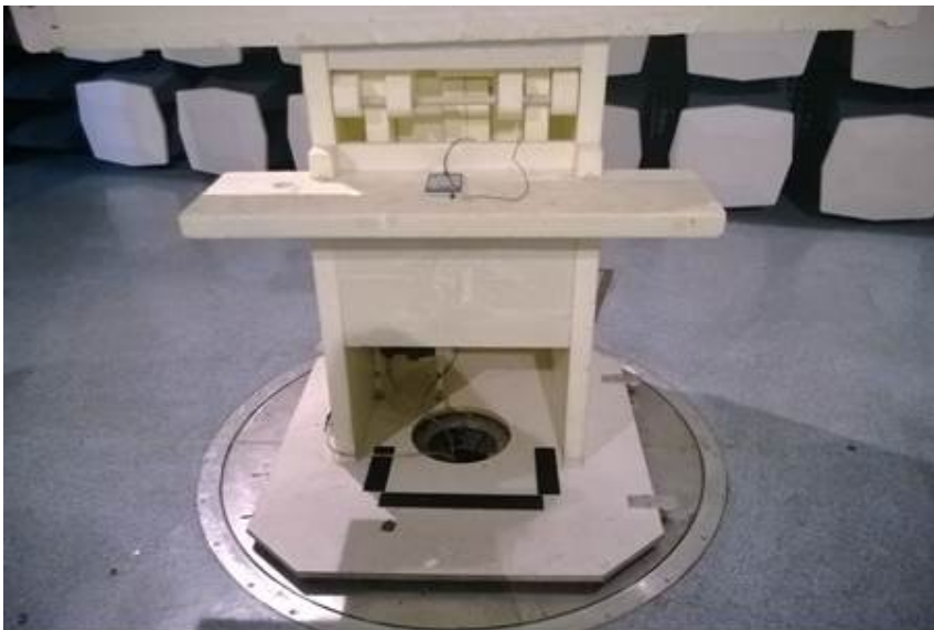
Picture 2. FCC Part 15B Radiated emissions
