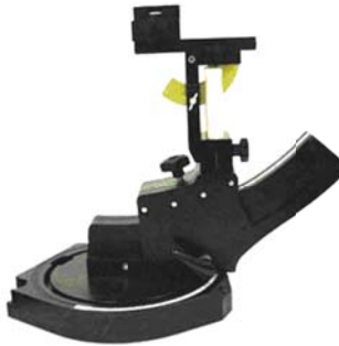
Device holder supplied by SPEAG
