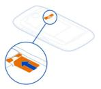
6 Line up the battery contacts, and insert the battery.
