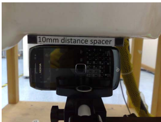
Photo of the device positioned for WR mode measurement – right edge facing phantom. The spacer was removed before the start of the measurements.
