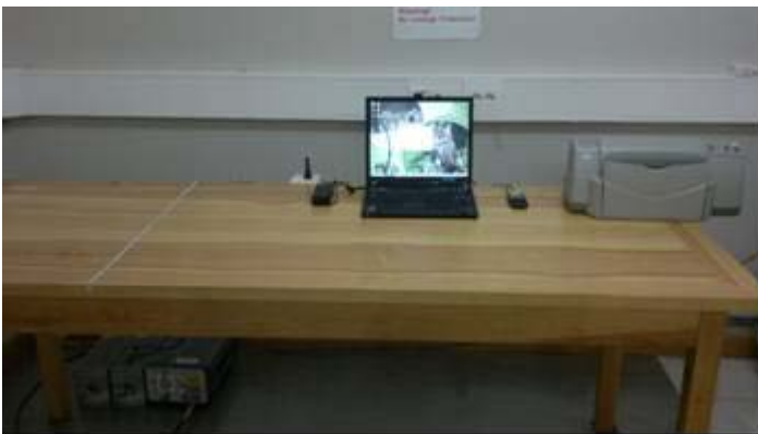
Picture 5. FCC Part 15B AC powerline conducted emissions, computer peripherals, measure from PC charger
