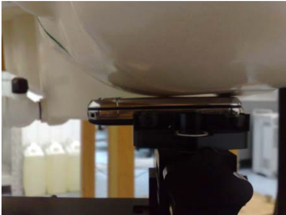
Photo of the device in “cheek” position with slide closed
