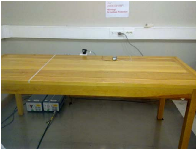
Picture 3 AC powerline conducted emission measurement 15C
