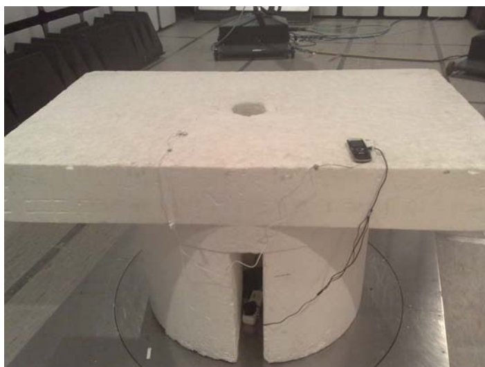
Picture 2 Radiated emission measurement GSM RX
