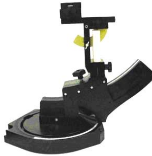
Device holder supplied by SPEAG
