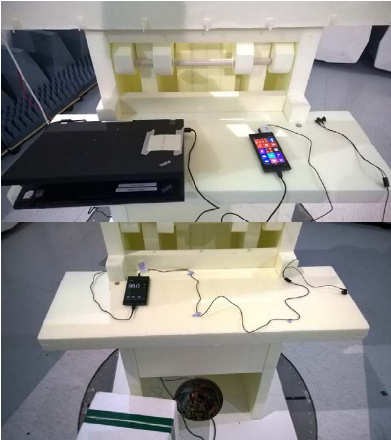
Picture 2. FCC Part 15B Radiated emissions
