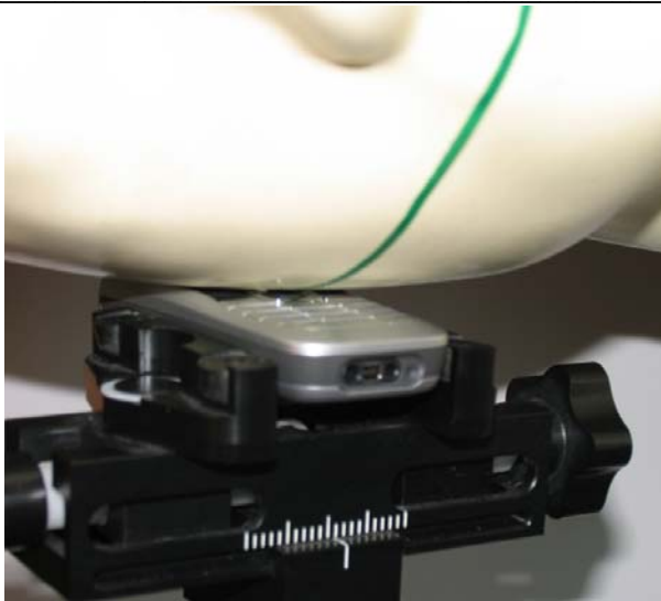
Photo of the device in "cheek" position
