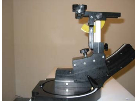
Device holder supplied by SPEAG
