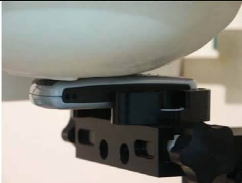
Photo of the device in “cheek” position
