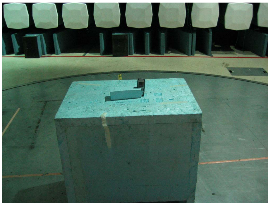
Photograph 1. Spurious radiated emissions test setup
