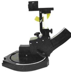
Device holder supplied by SPEAG
