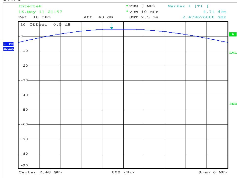
Modulation Type:  $\pi/4$  –DQPSK
