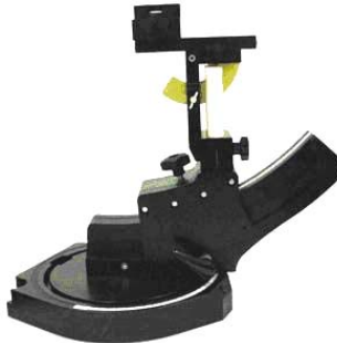
Device holder supplied by SPEAG
