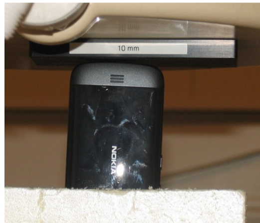
Photo of the device positioned for WR mode measurement – bottom edge facing phantom. The spacer was removed before the start of the measurements.
