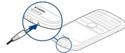
If you are using a USB charger, connect the charger plug to the USB connector.
