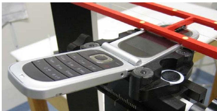
Photo of the device positioned under Test Arch
