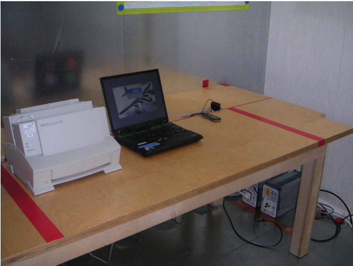
Picture 5 AC powerline conducted emission measurement GSM RX / Bluetooth TX / WLAN RX+ Computer peripherals
