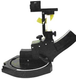
Device holder supplied by SPEAG
