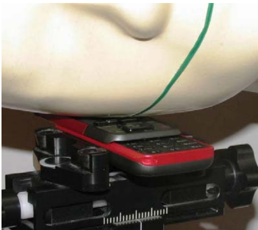
Photo of the device in "cheek" position with slide open
