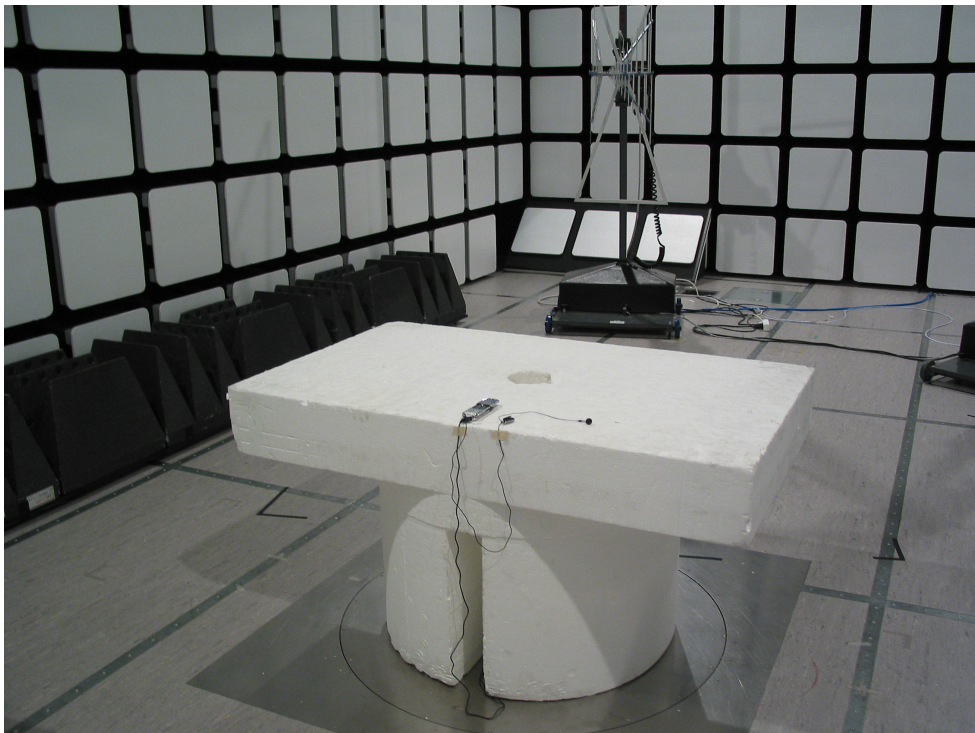
Picture 2 Radiated emission measurement
