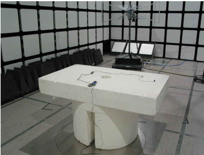
Picture 3 Radiated emission measurement GSM RX + FM radio on
