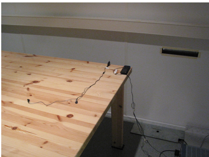
Picture 4 AC powerline conducted emission measurement GSM RX / FM radio on
