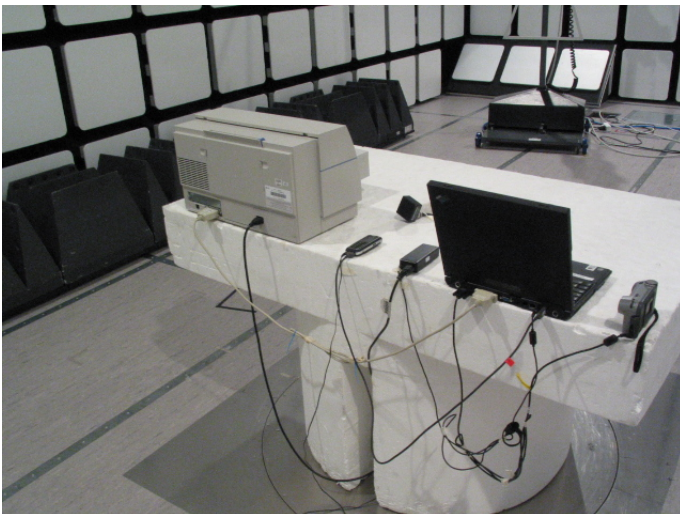
Picture 2 Radiated emission measurement GSM RX / Bluetooth TX + Computer peripherals
