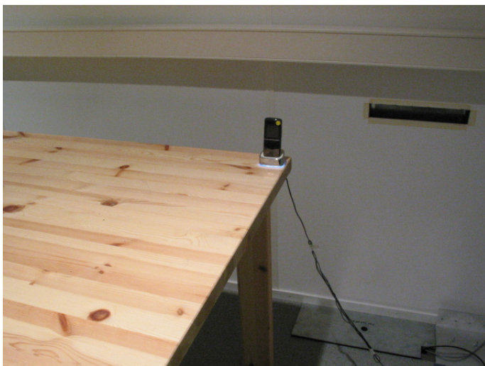
Picture 3 AC powerline conducted emission measurement desk stand GSM RX / Bluetooth TX
