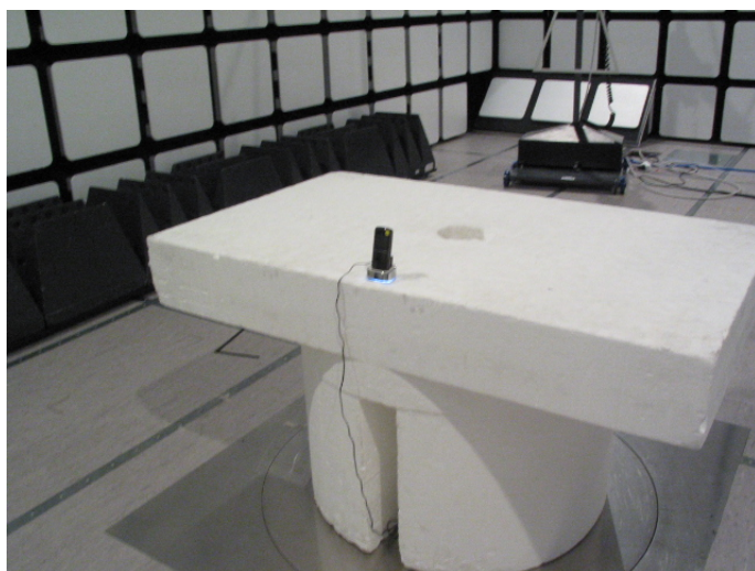
Picture 2 Radiated emission measurement with desk stand GSM RX / Bluetooth TX
